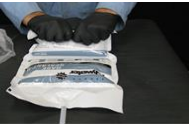
Burst primary seal
