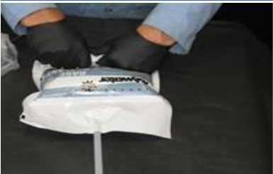
Bursting secondary seal
