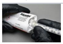
5. Place static mixer onto cartridge and lock into place by twisting clockwise. Depress handle on dispensing tool until PowerPatch comes out of mixing tip. Pump 1 or 2 more times to make sure you are getting an even mixture. Dispense and discard this excess material.
