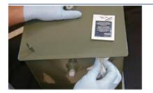
Clean area with cleaning wipe before applying sealant
